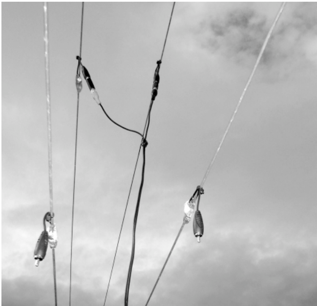
Figure 3 Piezo pickups attached to long wire instrument at WIRED Lab
