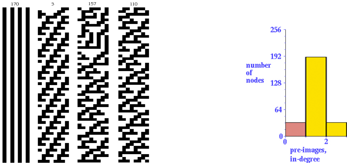
Figure 10: Spacetime plots of 8 cell rule 30 with decimal seed states indicated (left) and in-degree histogram, indicating a chaotic dynamic (right).
